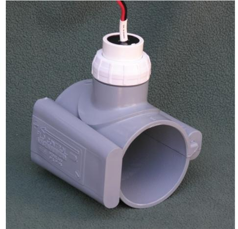
The flow sensor insert, held in place with a retaining nut, contains the detection circuitry and carries the unique four-bladed impeller on a transverse axle. The insert attaches to a housing that controls the location and alignment of the impeller. The housing is mounted in a PVC saddle therefore no additional mounting hardware is required. The axle and impeller along with the sealing o-ring are replaceable in the field.
