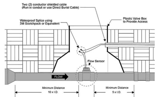
1. Always install with the flow arrow on the sensor pointed downstream. Allow 3 3/4" clearance to remove flow sensor insert from the saddle for service. The saddle is usually installed with the housing up in the vertical or 12:00 o'clock position. However, if necessary, it may be installed with sensor housing at an angle from vertical to provide clearance.
